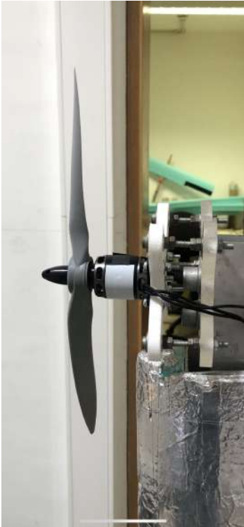
Figure 5.6: T-Motor AT2317 KV880 + APC 10" × 8" Sport assembly.
