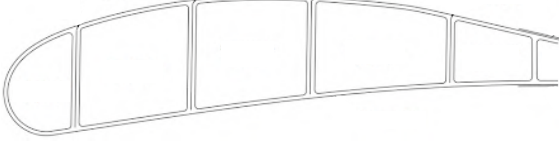
Figure 6: Section view of the CFRP flap. Adapted from [13].
