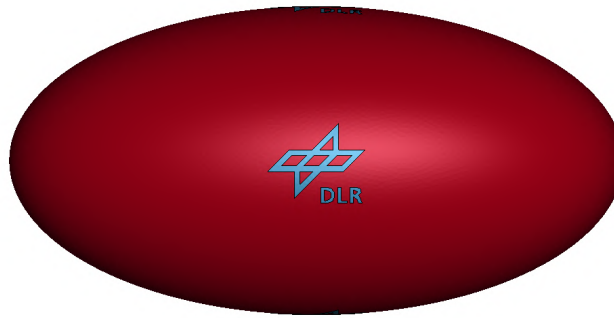
Figure 3.7: Bird Model in LS-DYNA.
