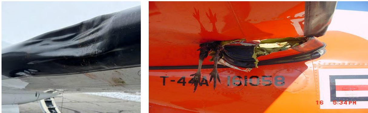
(a) Damaged wing leading edge of a BE-200 aircraft after impact with a Canada goose [7].
