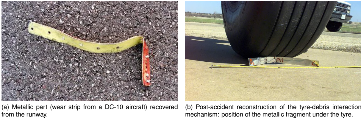
Figure 2.1: Technical evidence from the Concorde Air France flight 4590 investigation, illustrating the primary FOD and the reconstructed damage initiation sequence [27].
