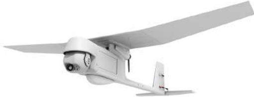
(d) RQ-11B Raven from AeroVironment that can be used to monitor and detect red tides
