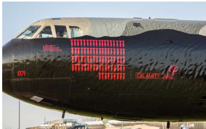
Figure 3.3: Airplane with fuselage skin that suffered buckling (Credit: Tony Webster, 2016)
