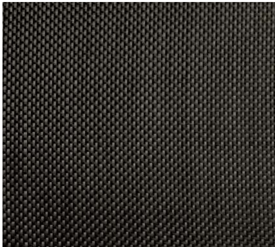
(a) Plain weave pattern trying to be modelled (Credit: EasyComposites)
