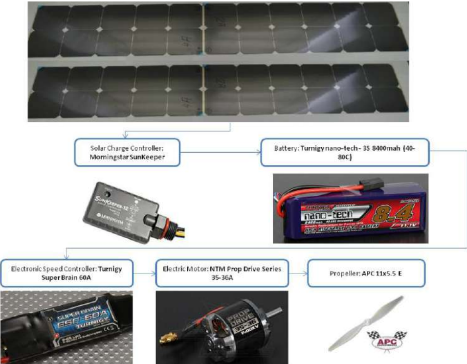
Figure 2.4: LEEUAV hybrid propulsive system scheme. [19]
