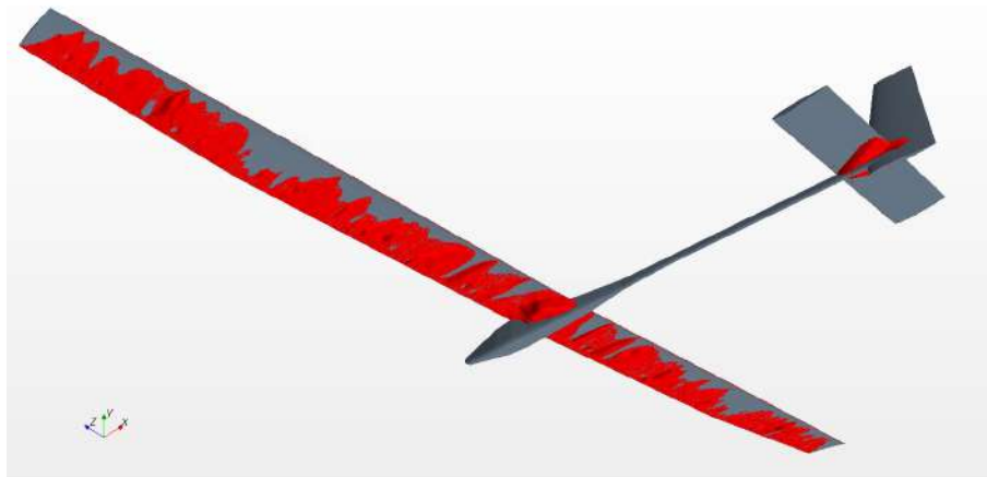
Figure 6.4: Spanwise lower laminar separation bubble, \text{AoA}=-10^\circ .
