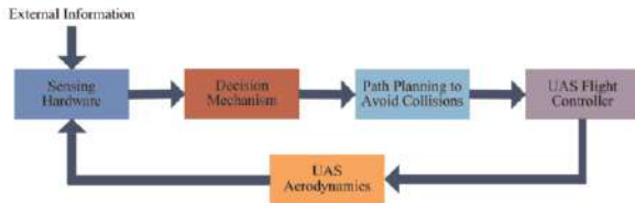
Figure 2: Architecture of an S&A system [15]
