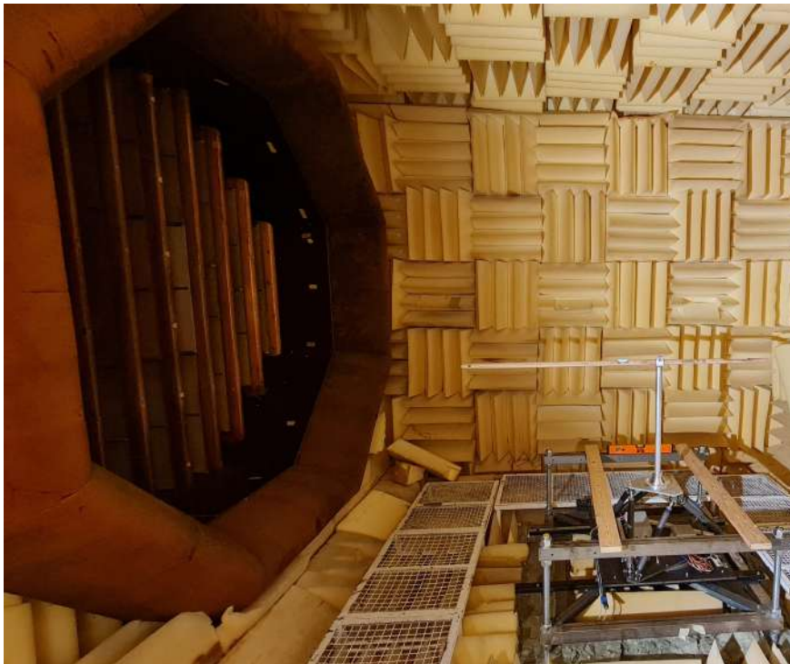
Figure 5.1: Positioning the Balance of Forces in the Wind Tunnel
