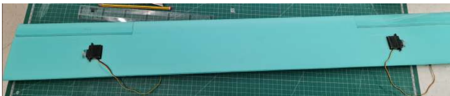
Figure 4.10: Installation of Servos Mechanisms
