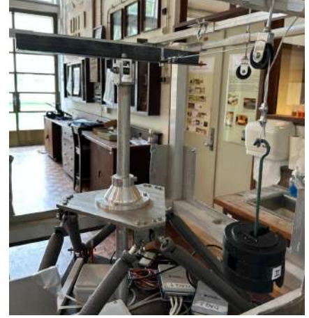
(b) -F_x with -M_z composed load case with approximately 30 N employed.
