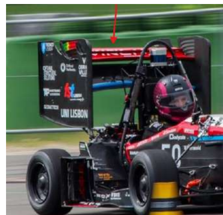
Figure 2.11: FST13's rear wing with DRS open.
