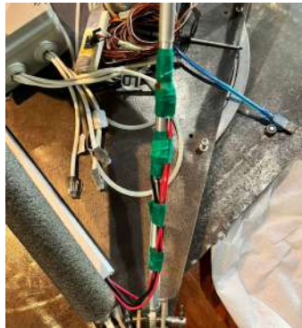
Figure B.5: Strain gauges welded to the respective cables.
