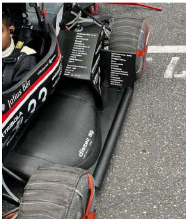
Figure 2.8: Example of the side diffuser assembly of a FS car (AMZ Racing).
