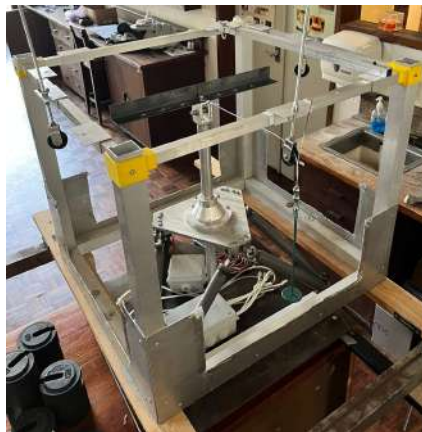
Figure B.9: Calibration apparatus with -F_x load case ready.
