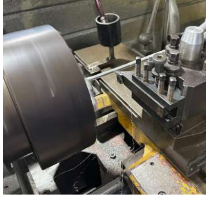
Figure B.2: Machining of the new sensing bar at LTO's lathe.
