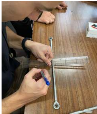
Figure B.3: Marking of the strain gauge's positions.
