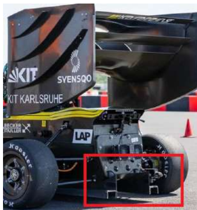
Figure 2.10: Example of a rear diffuser on a FS car (KA Raceing).
