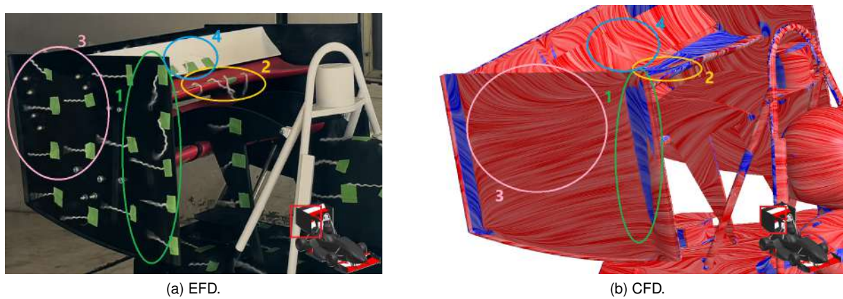
Figure 5.15: Flow visualization on rear wing upper surfaces and endplate.
