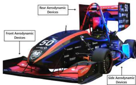
Figure 1.3: FST14's main aerodynamic devices.
