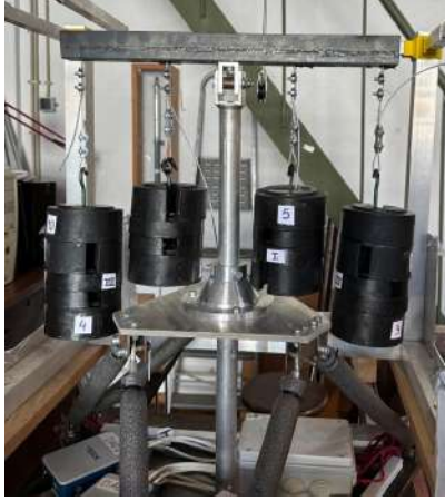
(a) -F_z load case with approximately 290 N in negative z direction. No moment created due to symmetrical loading.
