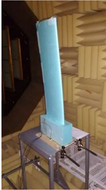
Figure 3.3: Baseline instrumented wing mount
