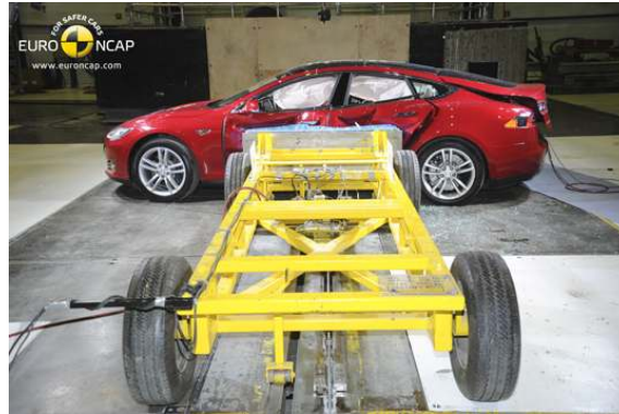
Figure 2.1: Side impact test on a Tesla Model S [13]
