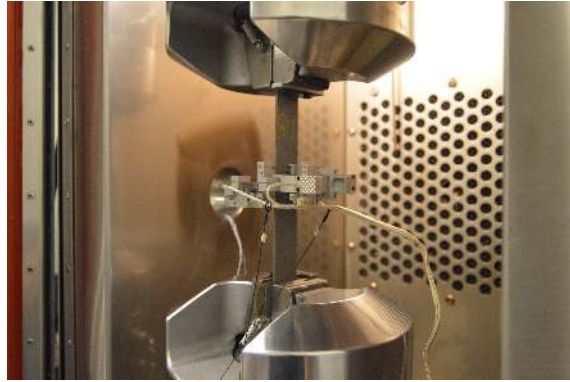
Figure 4.6: Tensile test apparatus
