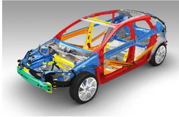
Figure 2.3: Volvo V40 safety cage [22]
