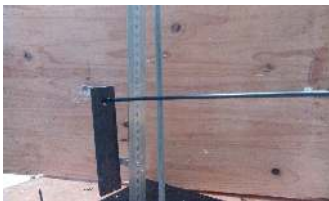
Figure 5.14: Setting used for the testing procedure of the carbon tube. Figure 5.15: Carbon tube with a weight at its free end.
