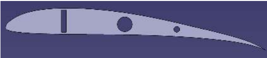
Figure 7.3: Rib CAD model, with the holes for the assembly to the spar, carbon tube, and passage of cables.
