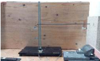
Figure 5.14: Setting used for the testing procedure of the carbon tube. Figure 5.15: Carbon tube with a weight at its free end.
