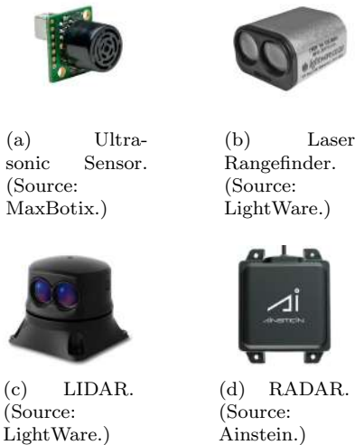
Figure 2: Active non-cooperative sensors.
