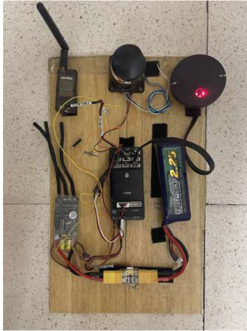
Figure 5.7: Assembly of the proposed layout (LIDAR-based obstacle detection system).
