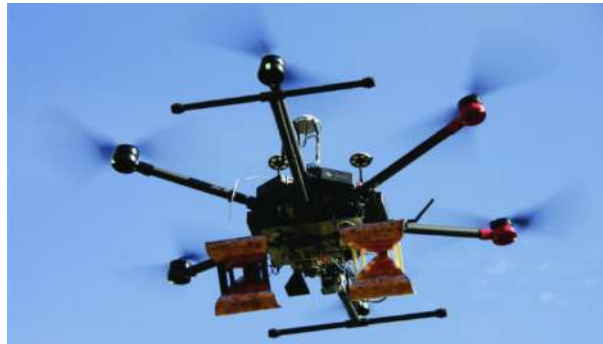
Figure 2.9: Measurement system with a GPSAR sensor module mounted below the UAV [43].
