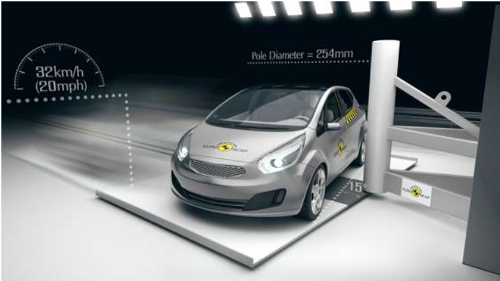
Figure 2.5: Pole side impact test [36]
