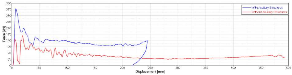
Figure 3.35: Force-displacement curves for effect of auxiliary structures
