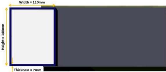
Figure 3.24: Structure front view
