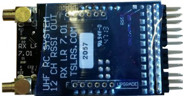
Figure 3.5: Long range radio receiver Thomas Scherrer Rx700. [71].
