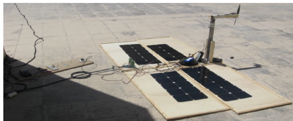
Figure 1.7: Assembly used to test the propulsion system [54].
