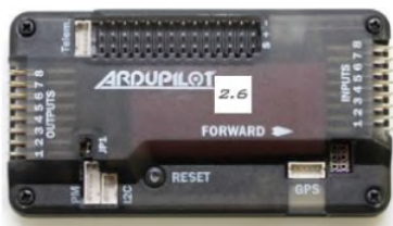
Figure 3.4: Autopilot Ardupilot APM 2.6 [70].
