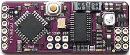
Figure 3.12: On-Screen Display MinimOSD from 3DR Robotics [75].
