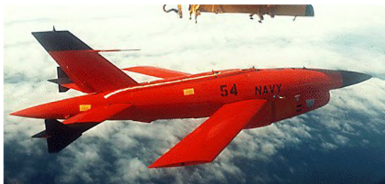
Figure 1.1: Jet-powered surveillance UAV Ryan Firebee [3].
