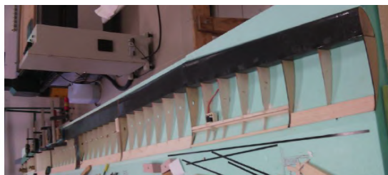
(a) Wing structure manufacturing.
