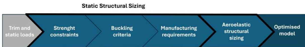
Figure 6.7: Structural sizing optimisation workflow.
