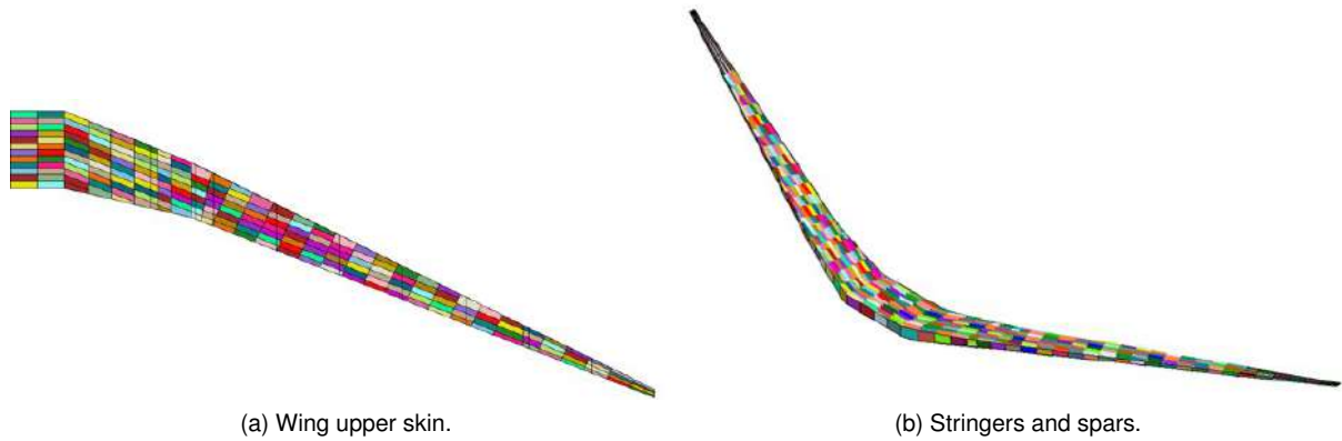
Figure 6.4: F25-AR15 wing upper skin, spars and stringers buckling fields.
