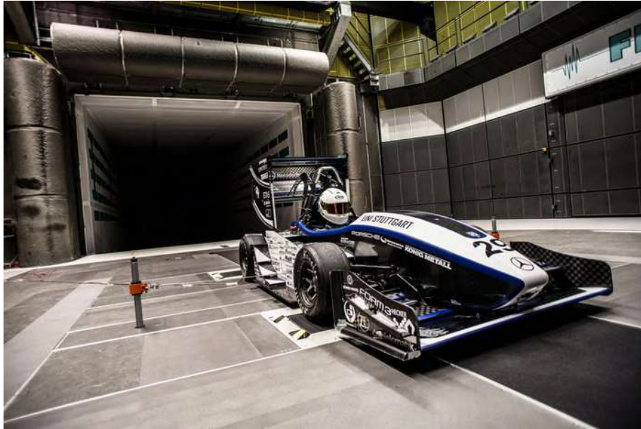
Figure 1.5: ReenTeam Uni Stuttgart wind tunnel testing to validate CFD and track data. From [5].
