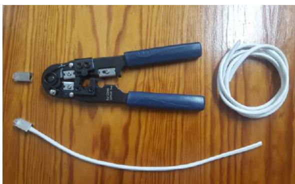
(a) Assembly of a generic RJ45 gate using a crimping plier.
