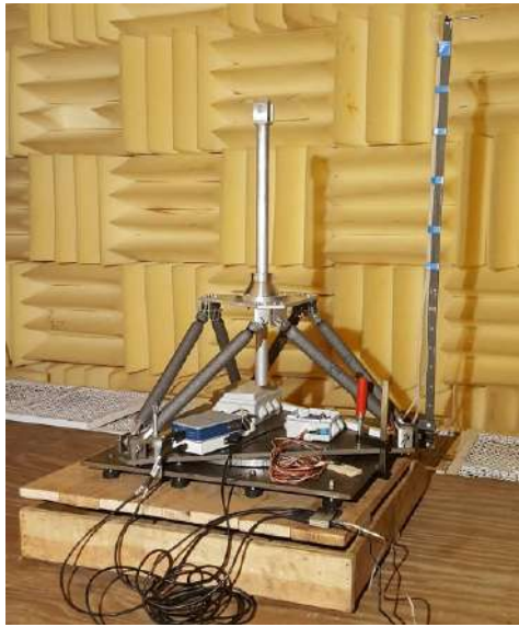
(a) Aerodynamic force balance set in wind tunnel test section.
