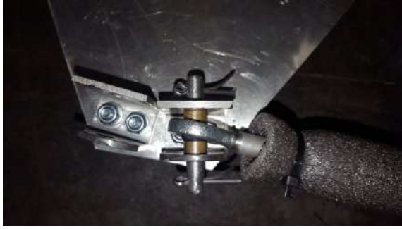
(a) Developed system to attach and fix the rod end bearing. (b) Apparatus with hoist to assemble the upper base with the sensing bars mounted.
