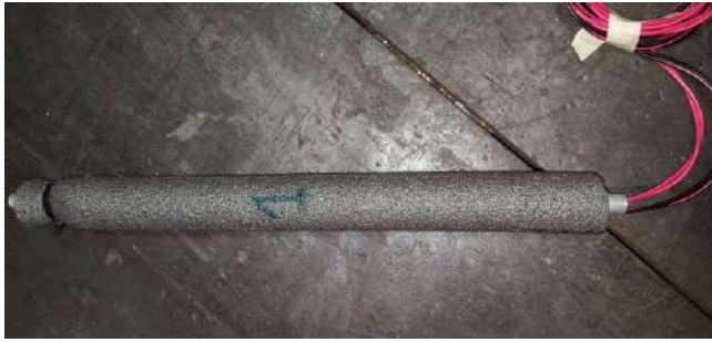
(a) Sensing bar coated with insulating tube.
