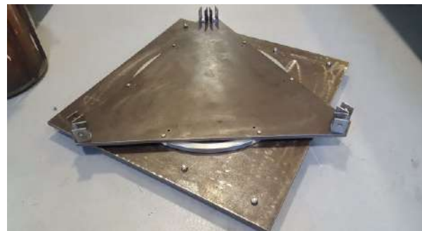
(b) Complete base with fixed platform and the 6 correspondent couplers.
