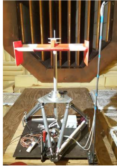
(b) Test model mounted on the force balance.
