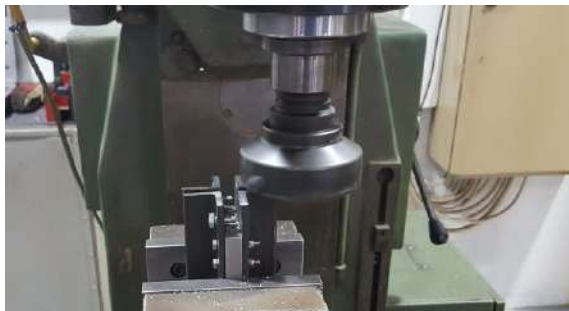
(a) Milling of the pitot support fixation.
