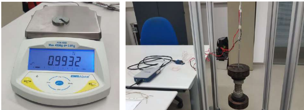
(a) Weighing of an increment weight to setup the load set.
