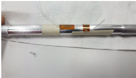
(c) Strain gauges glued to the sensing bar with paper tape to protect the wires output.
