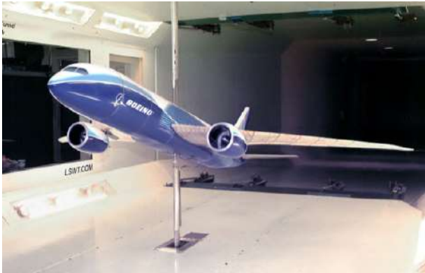
Figure 2.2: Aircraft model mounted on a force balance in wind tunnel tests. Courtesy of Boeing.
