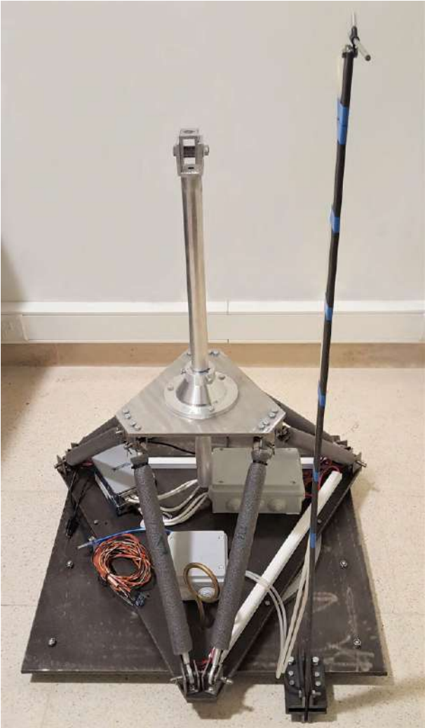
Figure 5.13: Aerodynamic force balance.
