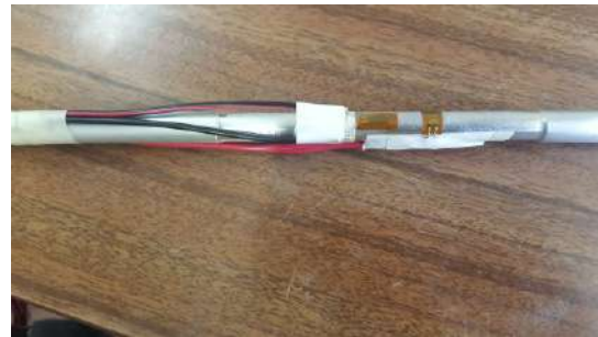
(d) Strain gauges with cables welded and fixed.
