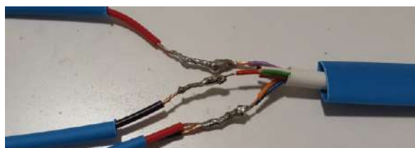
(b) Welding of strain gauge wires.
