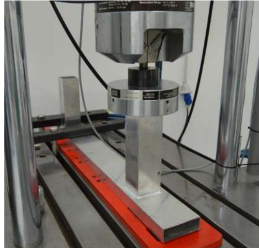
Figure 5.12: Final setup for the compression procedure
