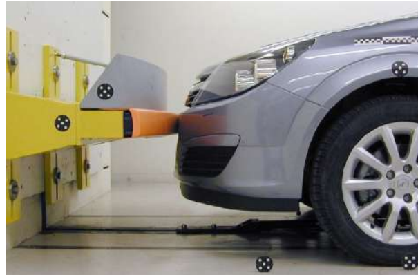
Figure 2.13: RCAR fixed bumper structure [55]
