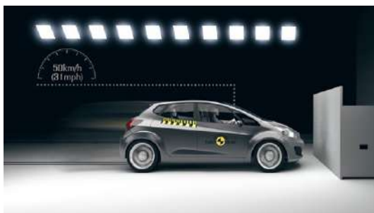
Figure 2.11: Fixed barrier NCAP front crash test [53]
