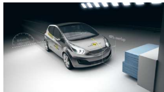
Figure 2.12: Deformable barrier NCAP 40% offset front crash test [53]
