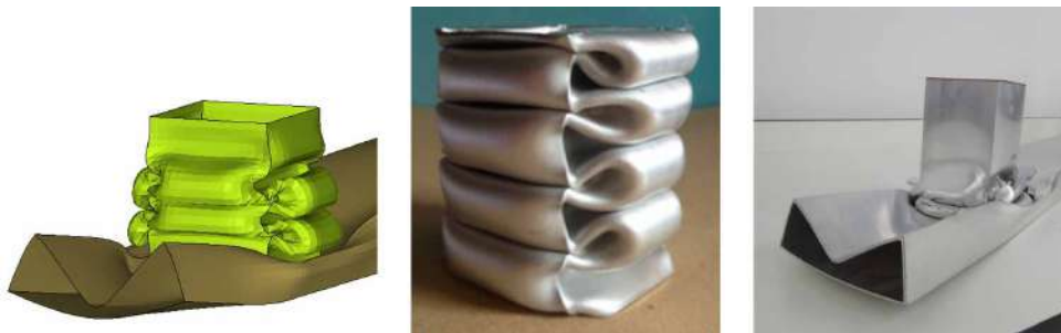
Figure 5.15: Comparison between the computational model, the expected result [81] and the obtained result
