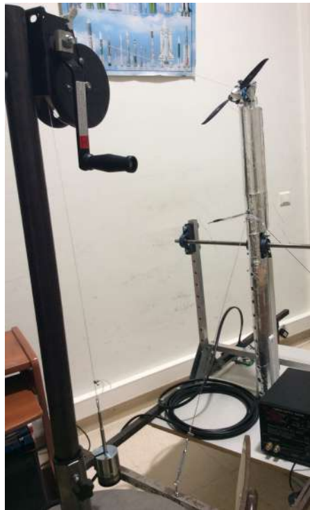
Figure 4.15: System used on the load cell calibration
