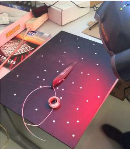
Figure 4.5: 3D scanning measurement of the blade
