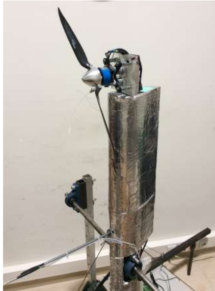
Figure 4.12: Resized support of the system motor+propeller
