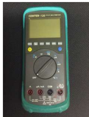
Figure 4.17: Multimeter used to perform the voltage sensor calibrations
