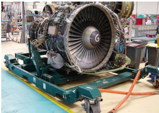
(a) CFM56-3 on engine stand.
