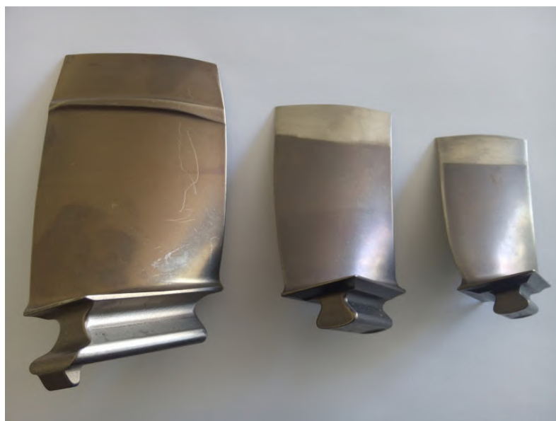
Figure 6.7: HPC blades from the first, second and third stages.
