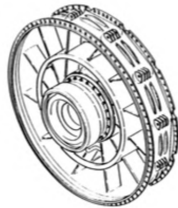
(b) Turbine Rear Frame.
