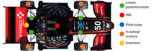
(a) Approximate location of the main instrumentation on FST14.
