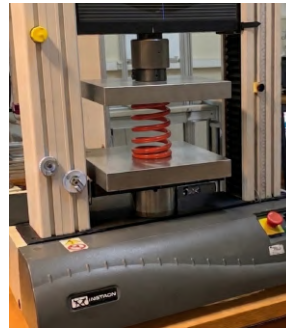
(a) Spring compression test.
