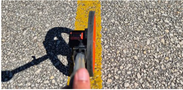
Figure 4.2: Track assembly using a measuring wheel (hodometer)
