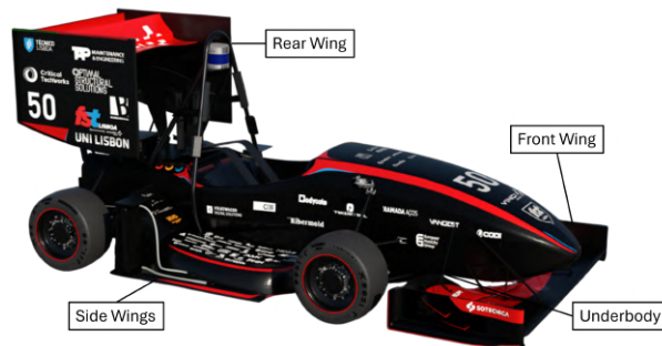
Figure 1.1: Aerodynamic elements of the FST14 prototype
