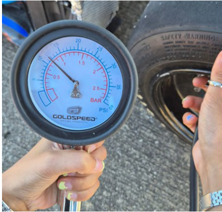
Figure 4.5: Tyre pressure monitoring using a handheld pressure gauge
