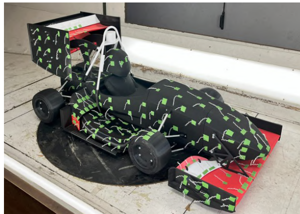
Figure 1.5: FST14 wind tunnel experimental campaign [8]
