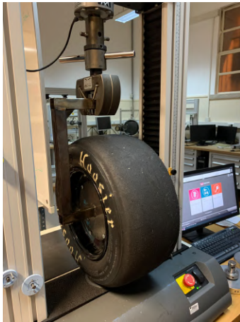
Figure 3.16: Instron 3369 UTM configured for quasi-static tyre vertical compression testing
