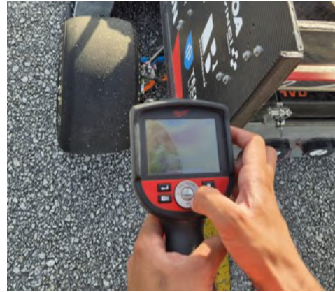
Figure 4.6: Tyre temperature monitoring using a thermal imaging camera
