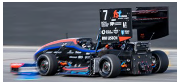
(b) Rear wing with DRS open [@FSG-Partenfelder]
