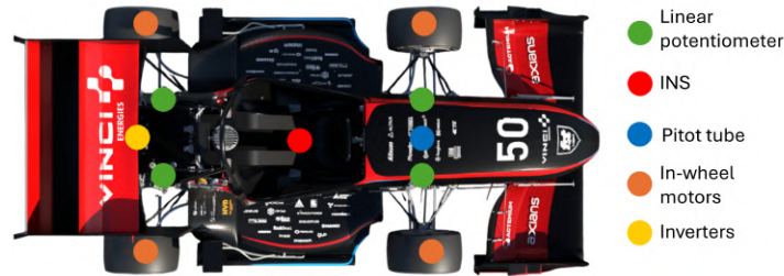
Figure 3.8: Schematic overview of the approximate mounting locations of the instrumentation used in the on-track campaign
