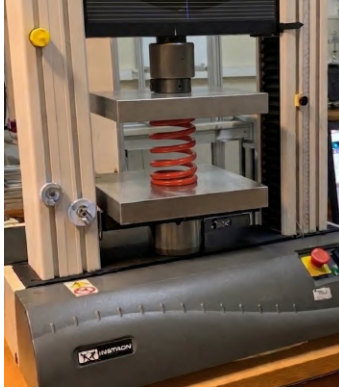
Figure 3.14: Instron 3369 UTM configured for quasi-static spring vertical compression testing
