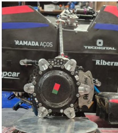
(a) Wheel-side assembly supported on stacked calibrated plates
