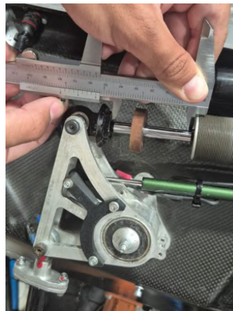
(b) Damper-stroke measurement using a caliper ruler
