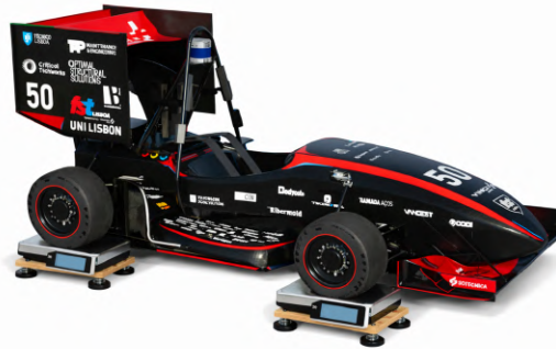
Figure 3.18: Vehicle positioned on corner scales during static setup
