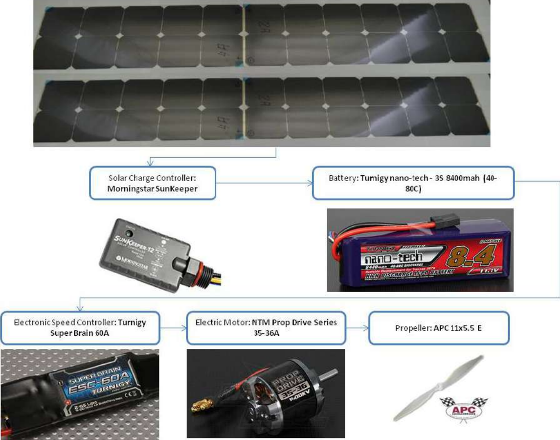
Figure 8.9: Scheme of the propulsion system components selected.
