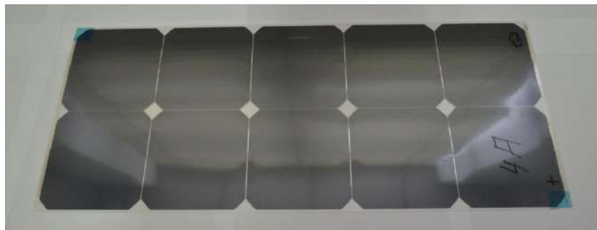
Figure 6.3: Solar panel using SunPower C60 cells in 2x5 array.
