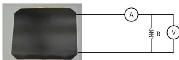
Figure 9.1: Test of an individual PV cell.
