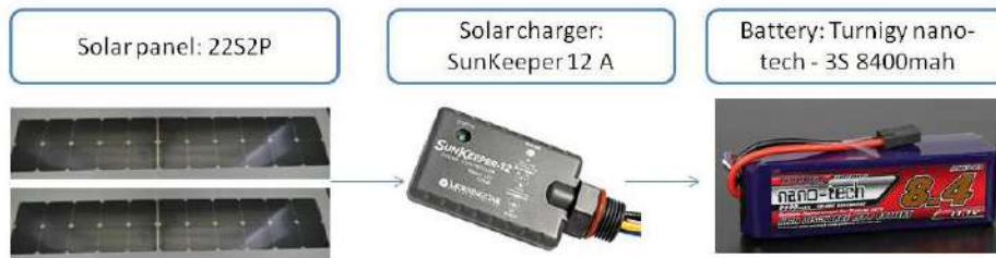
Figure 9.6: Experimental test of the solar charger controller.
