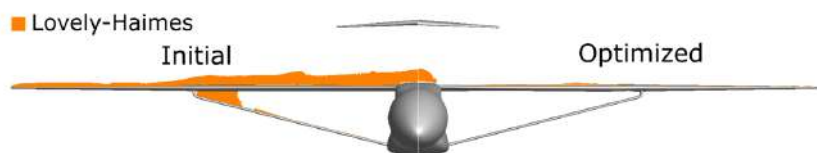
Figure 2.8: Optimized strut-braced wing. (Source: [33])
