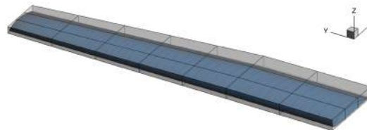
Figure 4.4: FFD box used to deform a wing surface mesh.
