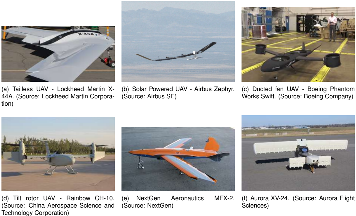
Figure 2.1: Some unusual UAV configurations.
