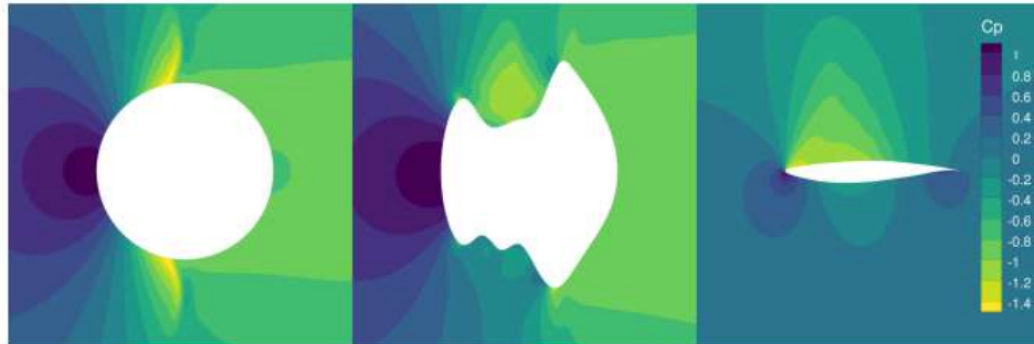
Figure 1.4: Aerodynamic optimization of an airfoil for transonic flow, starting from a sphere. (Source: MDOLab, University of Michigan)
