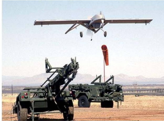
Figure 1.5: RQ-7 Shadow 200 launched from a hydraulic rail launcher [10].
