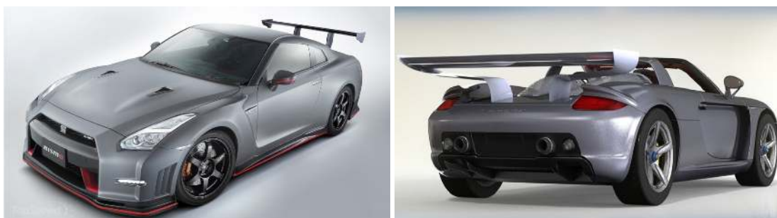
(a) 2015 Nissan GT-R Nismo equipped with a conventional design of rear wing. (Source: www.topspeed.com ) (b) 2007 Porsche Carrera GT equipped with the idealised proposed rear wing design.
