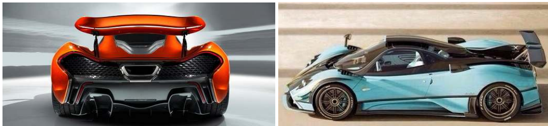
(a) 2014 McLaren P1 drag reduction system (DRS) rear (b) 2015 Pagani Zonda 760X front splitter, side skirts, canards, dorsal fin and multiple air intakes.
