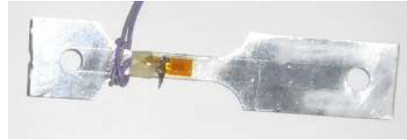
Figure 21: Built aluminium load cell with the strain gauge.
