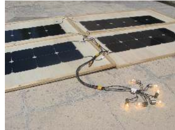
Figure 13: Full panel testing using light bulbs for load and a power meter for parameter measuring.
