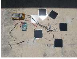
Figure 10: Circuit assembly used for the multiple cell tests.
