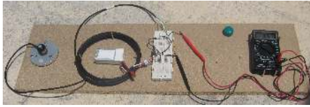
Figure 6: Solar irradiation measuring system.
