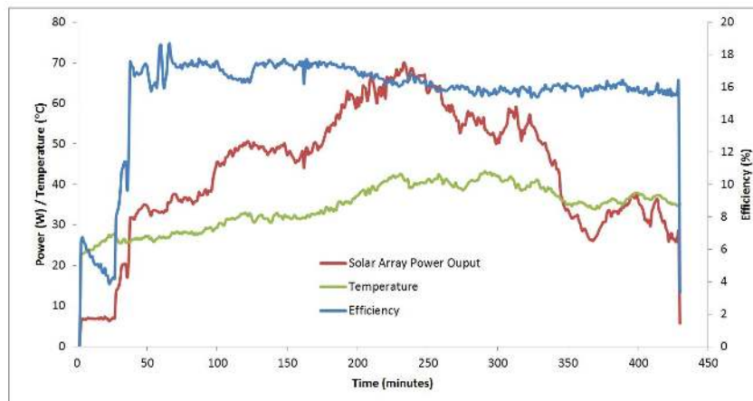
Figure 9.12: Energy generation sub-system power output, efficiency and temperature of the solar array during mission simulation.
