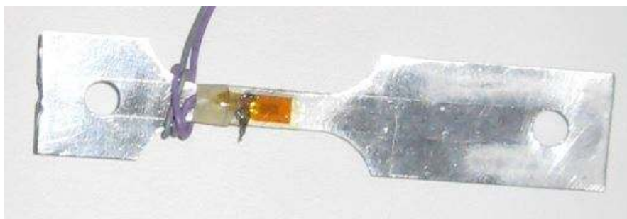
Figure 10.5: Built aluminium load cell with the strain gauge.
