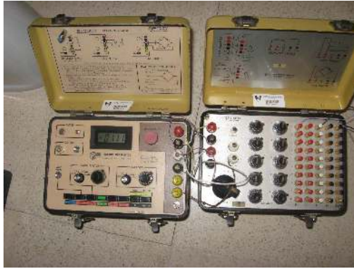
Figure 10.7: Strain indicator and dummy bridge used in the heat shrink film test.
