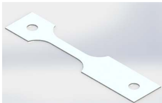
Figure 10.3: Final geometry of the aluminium load cell.
