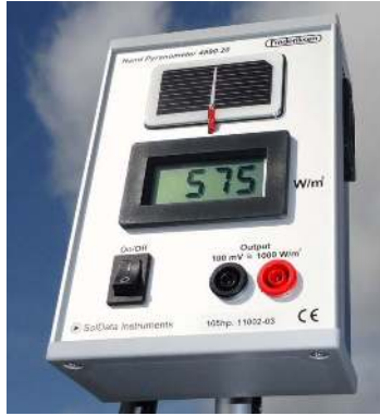
Figure 4.4: Photovoltaic cell pyranometer [Soldata, 2014].
