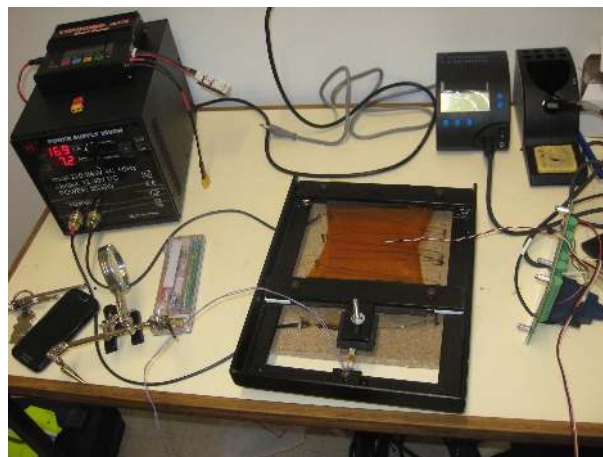
Figure 10.8: Heat shrink film test montage.
