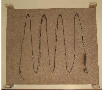
Figure 10.6: Heating element used in the heat shrink film test.
