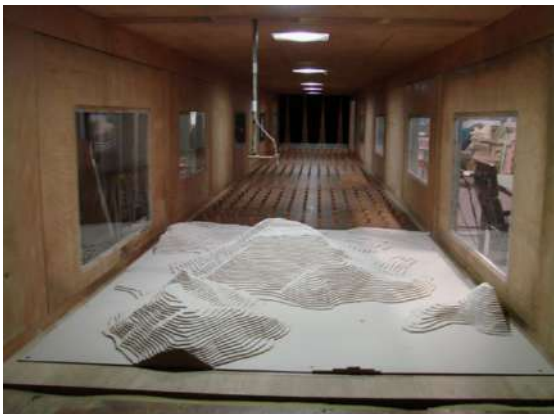
Figure 1.6: Realistic scaled model of the terrain for wind tunnel testing at Construction Aerodynamic Laboratory, Brazil [6]
