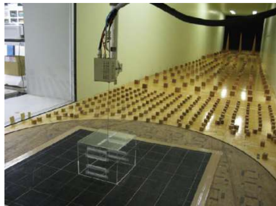
Figure 1.7: Wind tunnel set-up for concentration and velocity measurements (Niigata Institute of Technology) [7]
