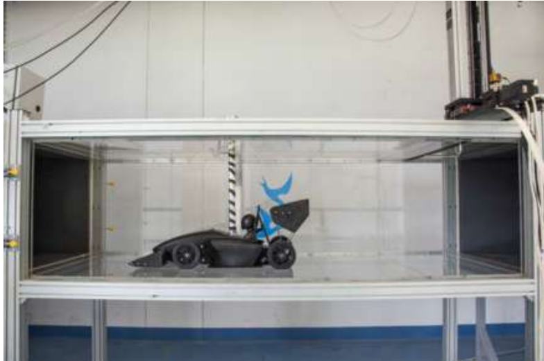
Figure 1.5: Experimental set-up of a scaled Formula SAE car [5]
