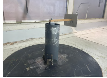
Figure 11: Rectangular flat plate mounted in the AWT.
