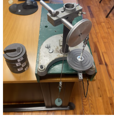
Figure 9: Load cell calibration setup.
