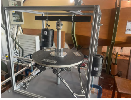
Figure 10: Force balance calibration setup.
