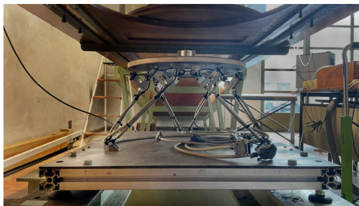
Figure 9.1: Force balance installation underneath the AWT.
