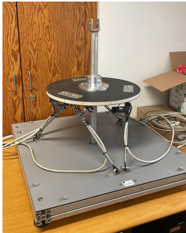
Figure 7.7: Final assembly of the force balance.
