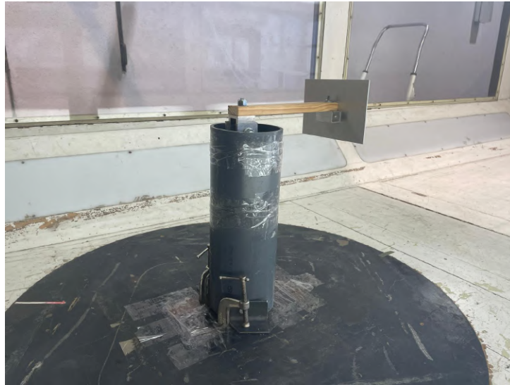
Figure 9.2: Rectangular flat plate mounted in the AWT.
