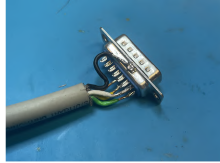
(b) Soldered connections on the DB15 male.
