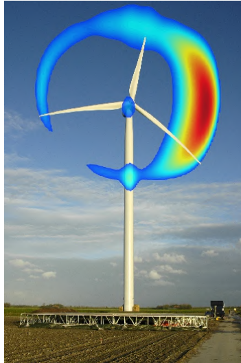
Figure 4.7: Representation of the acoustic map over a real HAWT [NLR, 2010]
