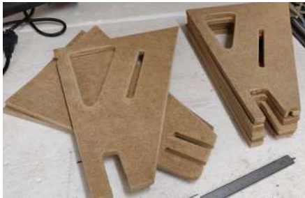
(d) Profiles after being polished
