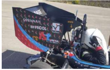
Figure 6.11: Wool tufts during testing day
