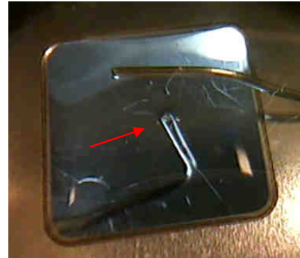
Figure 4: Liquid interface height achieved with the metallic foil with micro groove
