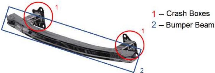
Figure 2.4: Complete aluminium bumper and crash boxes made from extrusions for the Renault Megane (adapted from [34])
