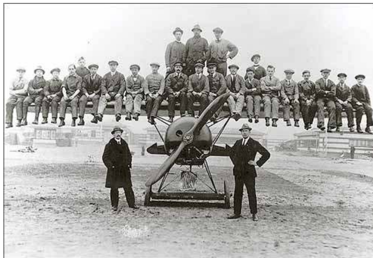
Figure 1.1: Picture of the Fokker D8 (or D VIII) used to demonstrate its strength [3]
