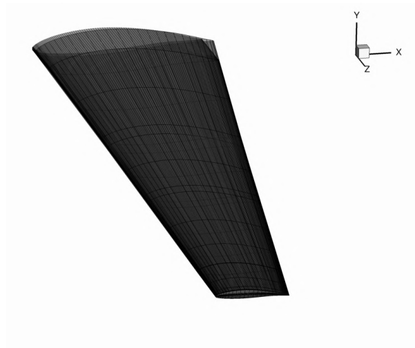
(b) Aerodynamic mesh for the L-23 wing geometry.
