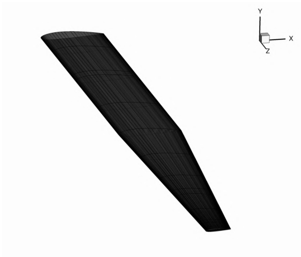
(a) Aerodynamic mesh for the semi-tapered wing geometry.
