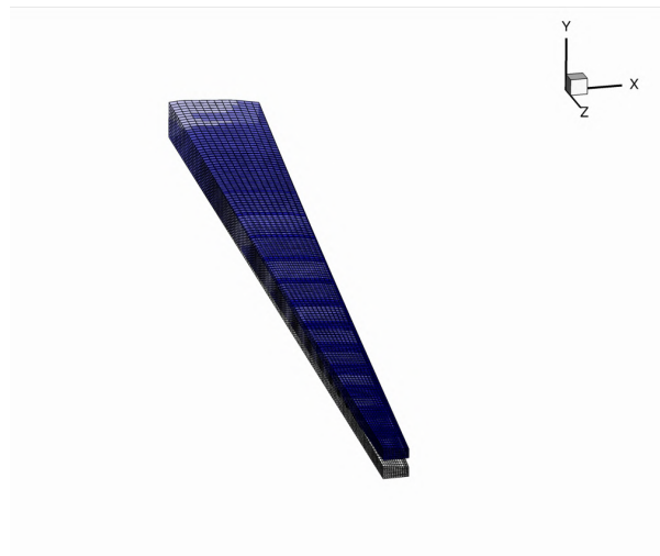
(d) Results for deformation of the wing structural layout, (outlined in the undisplaced structure).
