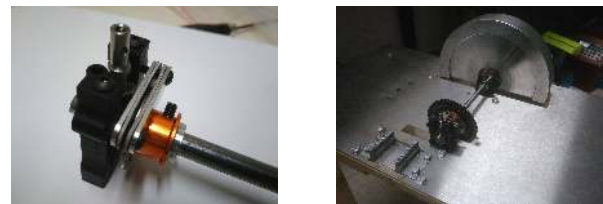
(a) Braking system. (b) Flywheel assembled.
