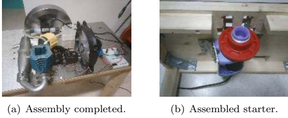
Figure 12: Test bench fully assembled.
