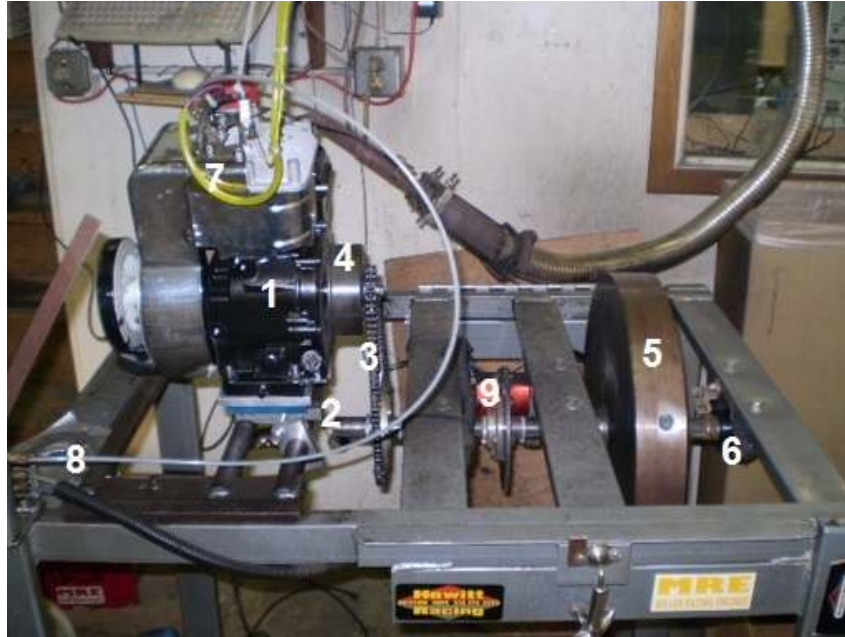
Figure 3.2: Components of an inertia dynamometer.
