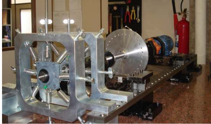
Figure 3.6: Balance equipment of flexible supports [17].
