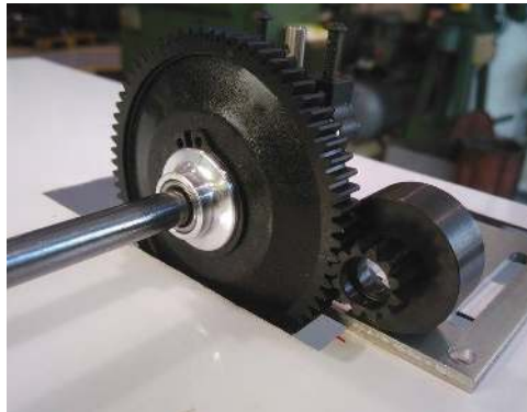
Figure 6.9: Composite spur gear.
