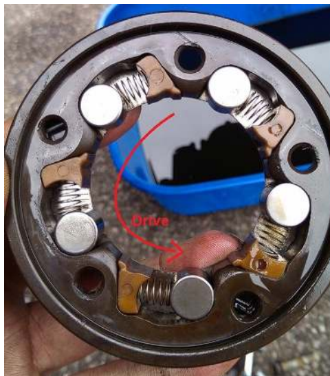
Figure 3.8: Outer ring of a trapped roller clutch (overrunning).
