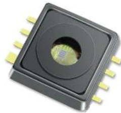
Figure 5.5: Pressure sensor KP236N6165.
