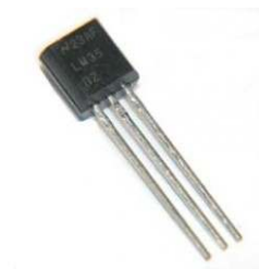
Figure 5.4: Temperature sensor LM35DZ.
