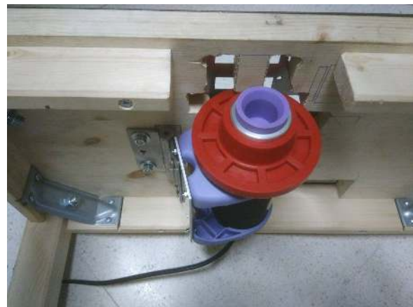
(b) Assembled electric starter.
