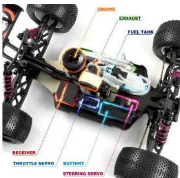
(a) Model racing car with assembled micro engine.
