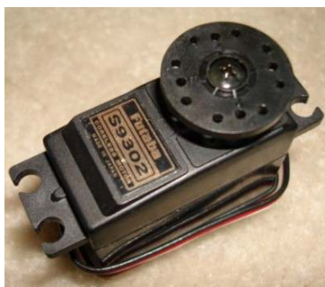
Figure 5.6: Electric servo for throttle and brake control S9302.
