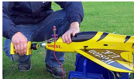
(b) Starting the Glow Plug engine of a model airplane.
