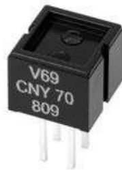
Figure 5.2: Rotation speed sensor (phototransistor).
