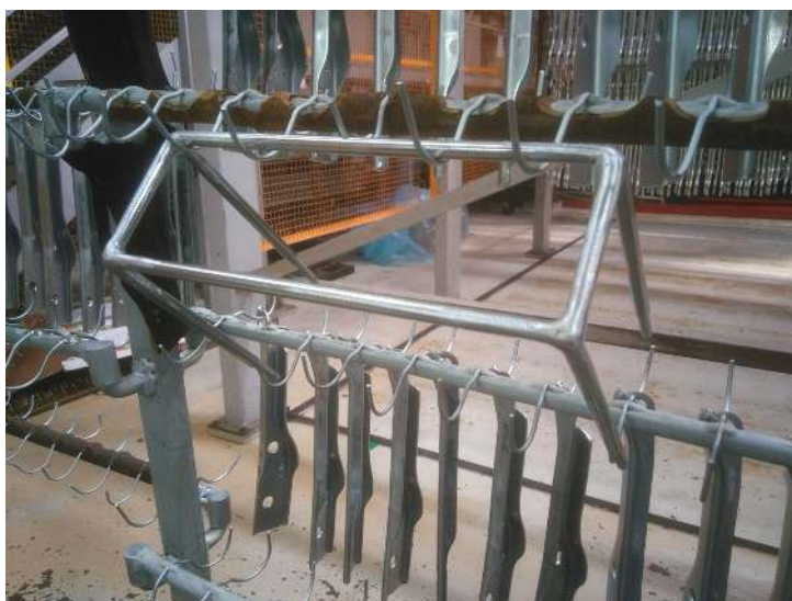
Figure 7.4: Flywheel safe after zinc plating in Electrofer IV.
