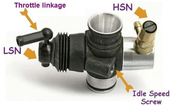
(b) Tuning parts of the carburetor.
