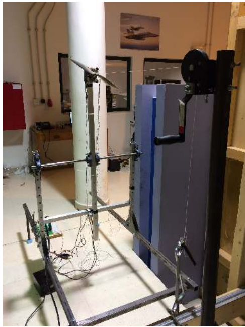
Figure 17: Structure used for the calibration of the load cell
