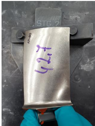
Figure 3: HPC blade measurement on the Go/NoGo tool
