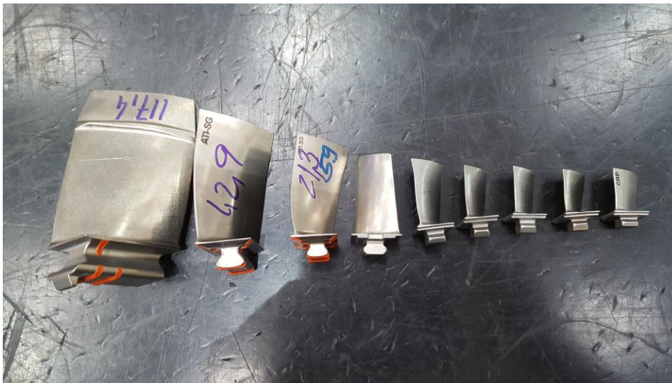
Figure 6.1: Blades from the CFM56-5B HPC: stage 1 to 9
