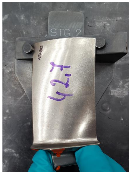
(c) HPC blade Measurement in the Go/NoGo tool
