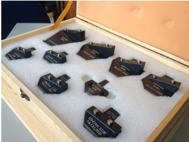
(a) Go/NoGo tool of the HPC blades for all stages
