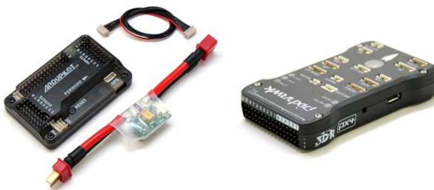
Figure 1.2: Popular open-source autopilots (ArduPilot Mega on the left (source: http://www.ardupilot.co.uk/ ), and Pixhawk on the right (source: pixhawk.org ))
