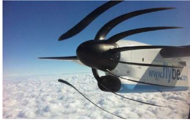
Figure 3.4: Distortion caused by a rolling shutter in the rotating blades of an airplane [80]
