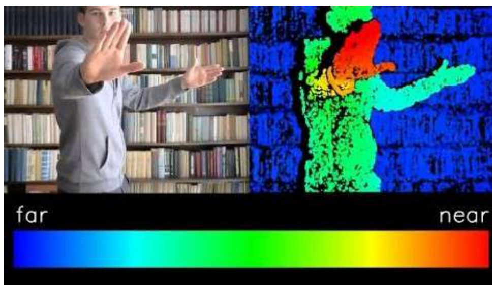
Figure 2.7: Depth map obtained from stereo vision [61]
