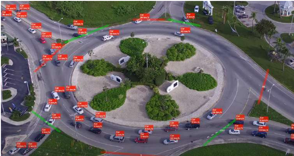
Figure 2.6: Vehicle tracking using UAVs equipped with vision sensors [57]
