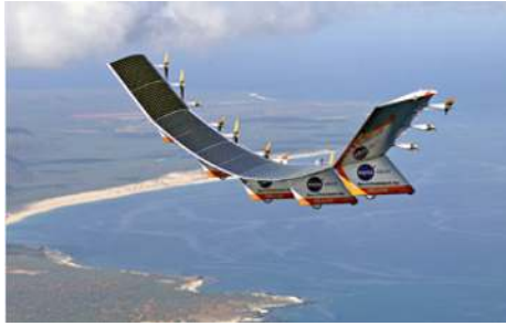
Figure 1.2: Helios aircraft showing large wing deflection [6].
