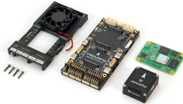
**Figure 2.** Flight controller Holybro Pixhawk RPi CM4 baseboard parts (from left to right): case with fan, baseboard, Pixhawk 6X, and Raspberry Pi CM4 [32].
