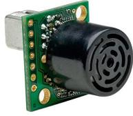
(a) Ultrasonic sensor. (Source: MaxBotix.)
