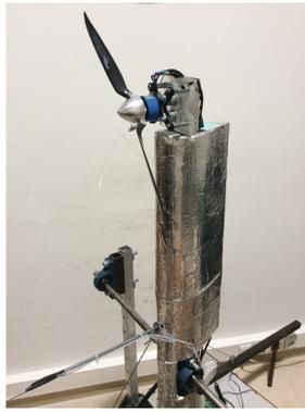
**Fig. 2.** Force balanced to characterize the motor+propeller system
